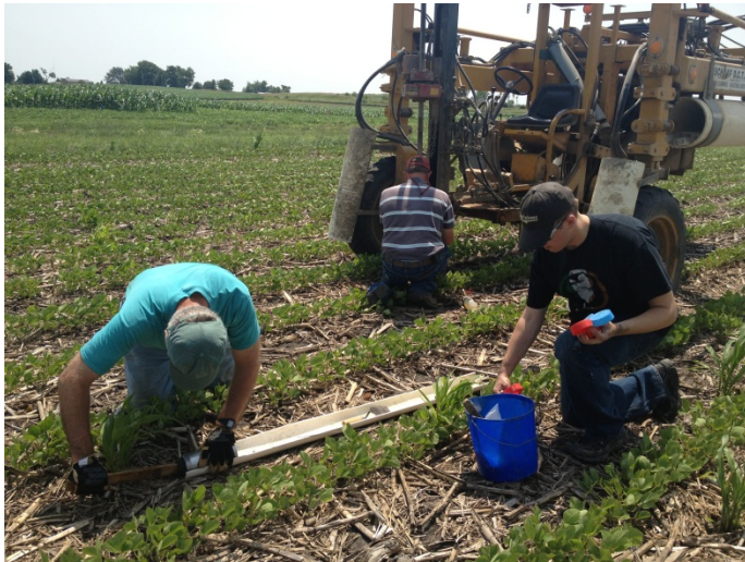
Intact soil core sampling for water retention analysis, July 2013, pictured from right to left ISU undergraduate Jacob House, Ben Knutson and Tom Kaspar of USDA-ARS. Photo credit: Andrea Basche
