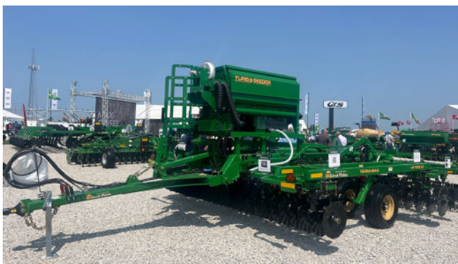
Figure 6. A vertical tillage tool with mounted air seeder box is a popular and efficient cover crop seeding method.
