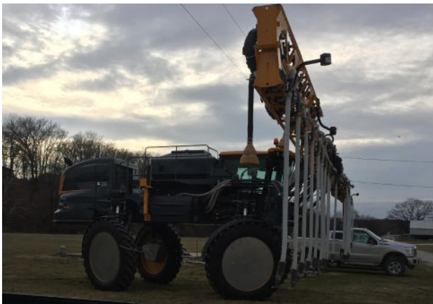
Figure 8. A modified sprayer outfitted with an air delivery seeding system on the boom.
