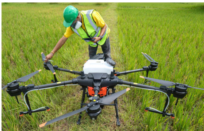
Figure 11. Large agricultural drones fitted with seeder attachments can broadcast cover crops in-season without crop damage in confined fields.
