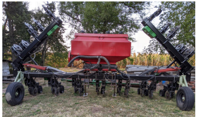
Figure 10. A row-unit based custom made interseeder equipped with an air delivery seed box. Photo courtesy of Jennifer Rees and University of Nebraska–Lincoln.
