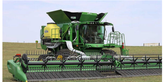
Figure 7. A air seeding box and tubing system mounted on a combine can seed cover crops at the same time as harvest.
